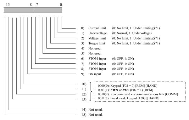
(\*1) Current limit, voltage limit and torque limit are the same as information in Type [21].
