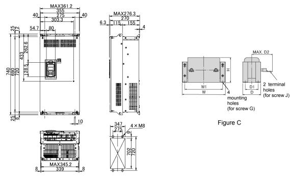
Approx. mass Reactor Figure WW1D D1 D2GН H1(kg) HD mode DCR4-75C M10 255 225 106 86 125 M6 (7\*13) 145 13 C LD mode DCR4-90C 255 225 116 96 140 M6 (7\*13) 145 M12 15
