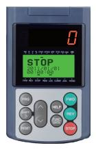
Figure 3.5-2 Display of the LED Monitor at Power-on
