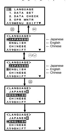
To display this menu screen, press the key in Running mode to switch to Programming mode.
