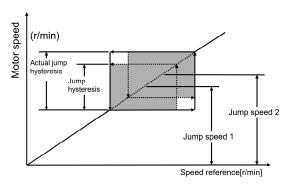
If the jump width is larger than twice the jump speed setting, the downward jump is limited at 0 r/min.
