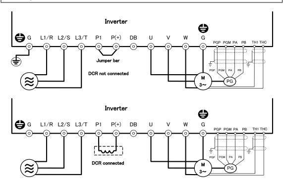
**Note:** In principle, the shielded sheath of wires should be connected to ground. If the inverter is significantly affected by external induction noise, however, connection to the common terminal (PGM, THC) may be effective to suppress the influence of noise.
