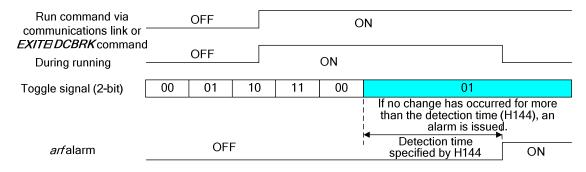
• During running, a toggle signal does not respond in the sequence of 00→01→10→11.
