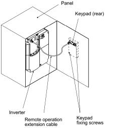
Figure 3.3-20 Mounting the Keypad on the Panel
