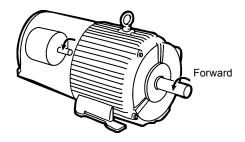
Figure 3.5-3 Forward Rotational Direction of Motor and PG
