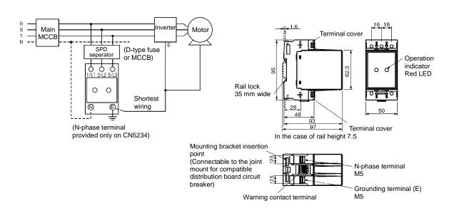
Figure 8.4 Arrester Dimensions and Connection Examples
