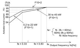
Activation level current and output frequency
