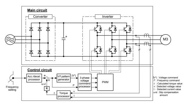
Figure 1.3.4 Speed Control Using the Slip Compensation Systems
