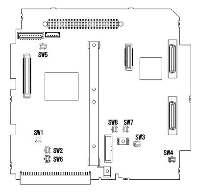
Figure 3.3-18 Location of the Slide Switches on the Control PCB
