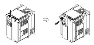
Figure 3.3-22 Removing a Keypad
