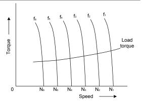
Figure 1.3.3 Speed vs. Torque Characteristics
