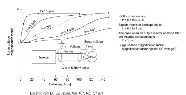
Figure C.2 Measured Example of Wiring Length and Peak Value of Motor Terminal Voltage
