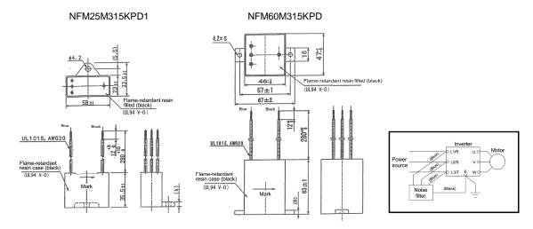
Figure 8.6 Filtering Capacitors Dimensions
