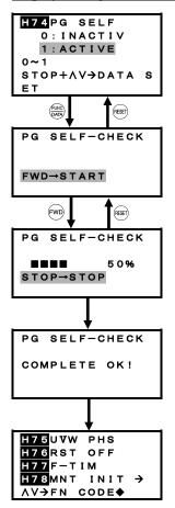
Change the data of the function code with the  $\bigcirc/\bigcirc$  keys.
