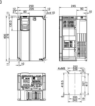
A figure given in the lower right-hand corner of each set of drawings shows the dimension of panel cutting required for employing external cooling. To employ external cooling for inverters of 30 kW or above, change the positions of the mounting bases. For details, refer to Chapter 3, Section 3.3.2 "Installing the Inverter, ■ When employing external cooling."
