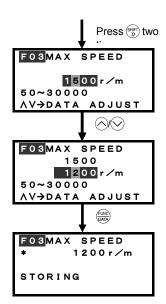
Change the function code data using the  $\bigotimes$  and  $\bigotimes$  keys. (In this example, change from 1500 r/min to 1200 r/min.)
