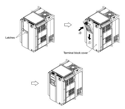
Figure 3.3-23 Mounting the Keypad
