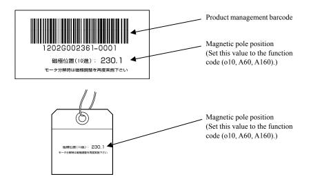
Figure 3.5-6 Magnetic Pole Position Offset Labels
