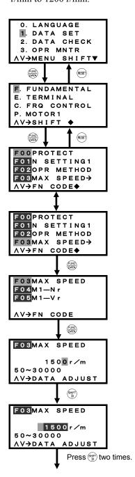
To display this menu screen, press the Running mode to switch to Programming mode. Move the cursor (flashing rectangle) at the left of the screen to "1. DATA SET" using the and keys. Then press the key to switch to the function code configuration screen.
