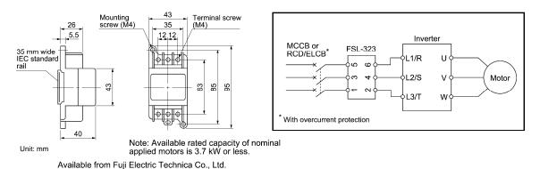
Figure 8.3 Dimensions of Surge Killer and Connection Example
