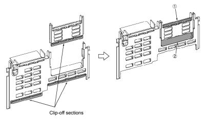
If the inverter output wire size is 22 mm², remove clip-off section 1; if it is 38 mm², remove clip-off section 2 before wiring.
