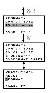
Change the time format data using the  $\bigcirc$  and  $\bigcirc$  keys.
