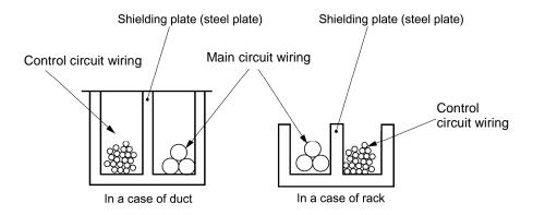
Figure A.7 Separate Wiring
