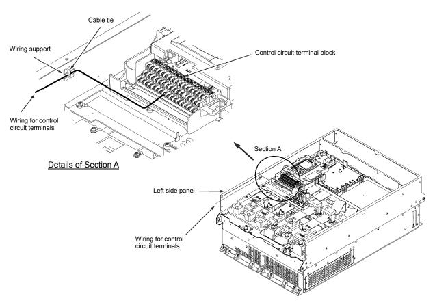
Figure 3.3-17 Wiring Route and Fixing Position for the Control Circuit Wires
