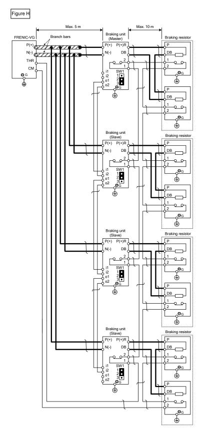
Note 1: For DB160V-41C, two braking resistors are used per one unit.
