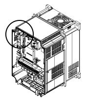
③ Connect the battery cable to the connector CN7 on the control printed board.
