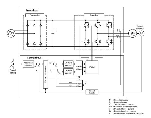
Figure 1.3.7 Example Vector Control Architecture
