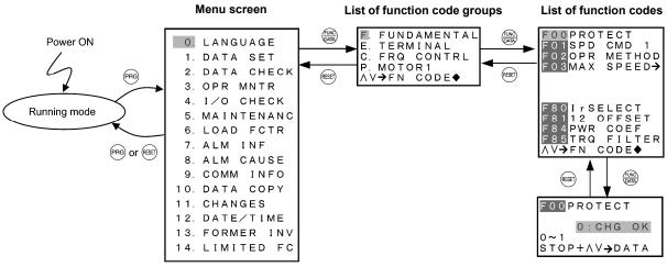
Figure 3.4-8 Configuration of Screens for "DATA SET"
