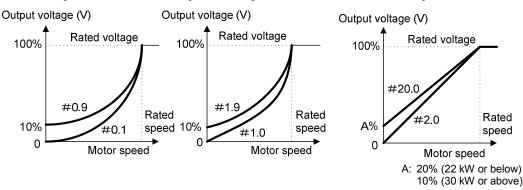
**Note:** When replacing the VG7 (22 kW or below) with the VG1, specify the torque boost according to the torque boost conversion table in Chapter 12, Section 12.5.
