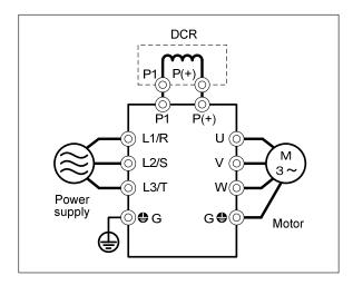
Figure 8.9 External View of a DC Reactor (DCR) and Connection Example
