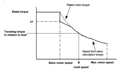
k1 indicates the motor torque determined from H66 (Rated load) and H62 (Rated lifting speed). The motor speed is limited by the base speed with the loads exceeding the rated load. The rated motor torque can be operated, using H64, H203, H206, H209, H212 (Safety coefficient).
