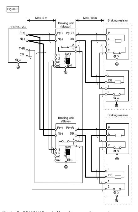
Note 1: For DB160V-41C, two braking resistors are used per one unit.
