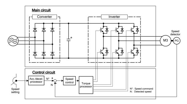
Figure 1.3.5 Closed-loop Speed Control: Basic Architecture
