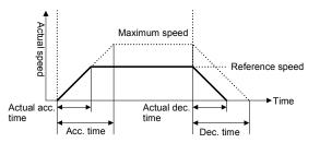
Writing data to S08 (Acceleration time) or S09 (Deceleration time) via the communications link (RS-485, T-Link, SX-bus, or fieldbus) automatically copies the data to F07 or F08 as is, respectively.
