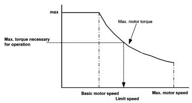
The limit speed is obtained from the relationship between the maximum motor torque and maximum torque necessary for acceleration/deceleration. The maximum motor torque can be operated, using H64, H203, H206, H209, H212 (Safety coefficient).
