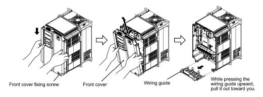
Figure 3.3-4 Removing the Front Cover and the Wiring Guide (FRN11VG1□-2□)
