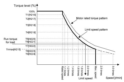
H225: Limit speed discrimination interval (start speed), H226: Limit speed discrimination interval (end speed)
