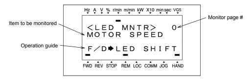
Figure 3.4-5 LCD Monitor Sample Detailed for the LED Monitor Item
