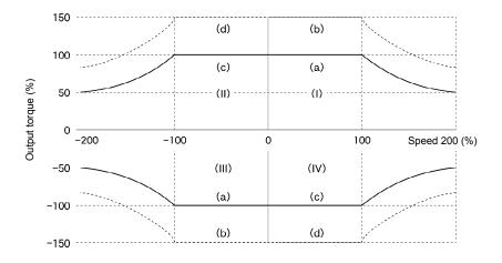
Figure 9.1 Output Torque Characteristics (HD mode)
