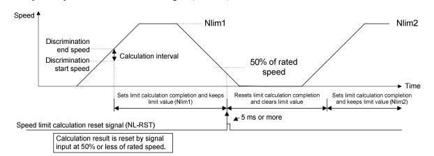
Each time the polarity of the speed command value changes (hoisting lowering), the limit speed is calculated when acceleration takes place, regardless of the speed limit calculation reset signal (NL-RST).
