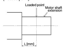
The maximum allowable value of radial load applied by the belt is shown in the figures below. The data is classified by the frame number and the rotation speed. If the point which is decided by the radial load FA (kN) acting on the motor shaft and the length L (mm) from the stepped joint at shaft end to the center of the pulley (the distance to the FA load points) is within a curve, the motor can be operated by that pulley. Refer to the technical leaflet of the induction motor for the details.
