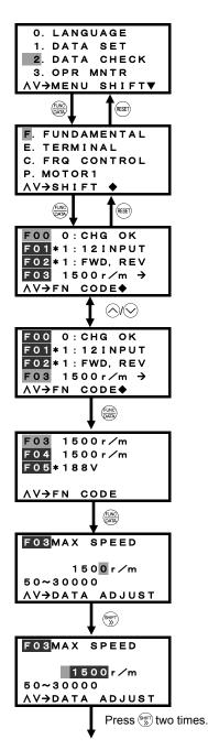
To display this menu screen, press the key in Running mode to switch to Programming mode. Move the cursor (flashing rectangle) at the left of the screen to "2. DATA CHECK" using the and keys. Then press the key to switch to the function code configuration screen.
