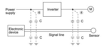
Figure A.5 Electrostatic Induced Noise
