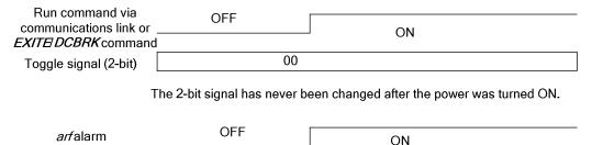
**Note:** When the power is turned ON, a run command is entered with the start of toggle signal monitor, an alarm //-/- is issued. Therefore, enter a run command after at least one cycle of toggle signal like  $00\rightarrow01\rightarrow10\rightarrow11$ .
