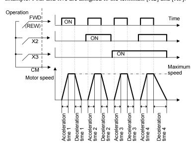
\* If you switch the acceleration/deceleration times, the ASR constants and S-curve actions are switched simultaneously. You can see which set is currently selected from (1, 2, 3, 4) on the "I/O check" screen of the KEYPAD panel. When the data set 3 is selected, "■PARA3" is indicated on the display.
