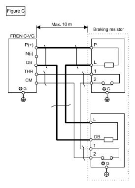
Note 1: For DB160V-41C and DB200V-42C, two braking resistors are used per one unit.
