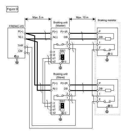
Note 1: For DB200V-41C, DV220V-41C, DB200V-42C and DB220-42C, two braking resistors are used per one unit
