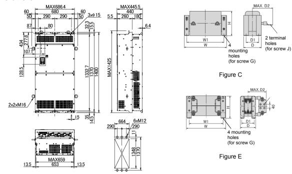
Approx. mass Reactor Figure W W1 D D1 D2 G Н H1 (kg) DCR4-315C 400 345 M10 (12\*22) 225 HD mode C 146 118 200 M16 40 MD mode DCR4-355C 400 345 156 128 200 M10 (12\*22) 225 4\*M12 49 E LD mode DCR4-400C 445 385 145 117 213 M10 (12\*22) 245 4\*M12 52
