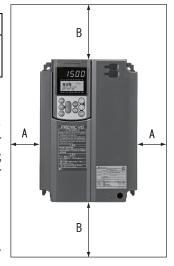
Figure 3.3-1 Mounting Direction and Required Clearances
