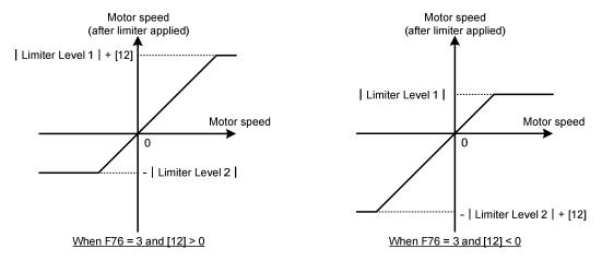
Input voltage for [12] is  $\pm$  10V at the maximum motor speed (  $\pm$  100% ).
