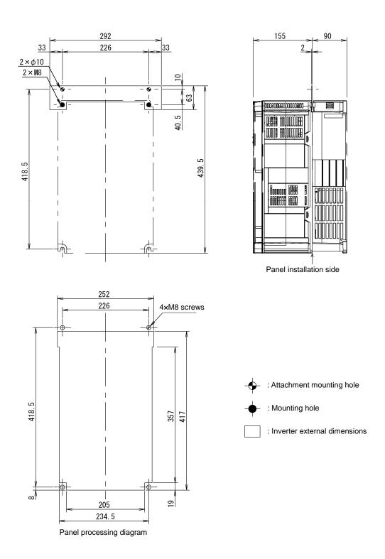
Figure 8.13 External Cooling Attachment External Dimensions (continued)
