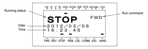
Figure 3.4-3 Display of Running Status
