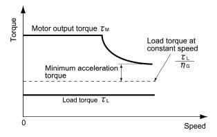
Figure 9.3 Example Study of Minimum Acceleration Torque
