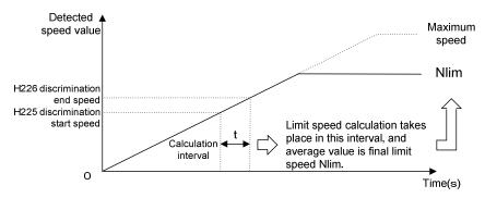
Within the calculation interval, the limit speed is calculated from the torque command that occurs and the instantaneous value of the acceleration data. When the speed reaches the limit completion speed, the average value of the calculated results is used as the final limit speed.
