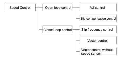
Figure 1.3.1 Classification of Speed Control Systems
