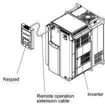
Figure 3.3-21 Using the Keypad Remotely in Your Hand
