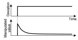
You can use D: differential time as a parameter to determine the effect of D control action. A large differential time attenuates an oscillation caused by P control action quickly when a deviation occurs.
