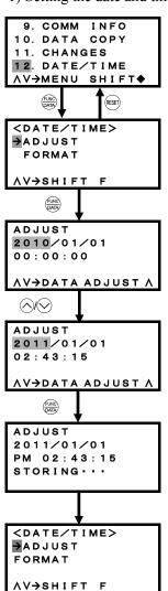
To display this menu screen, press the (PRO) key in Running mode to switch to Programming mode.
