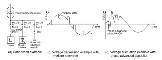
• Use a DCR when the interphase voltage unbalance ratio of the inverter power supply exceeds 2%.
