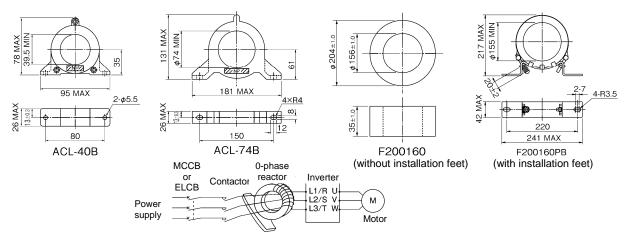
Figure 8.12 Dimensions of Zero-phase Reactor for Reducing Radio Noise (ACL) and Connection Example
