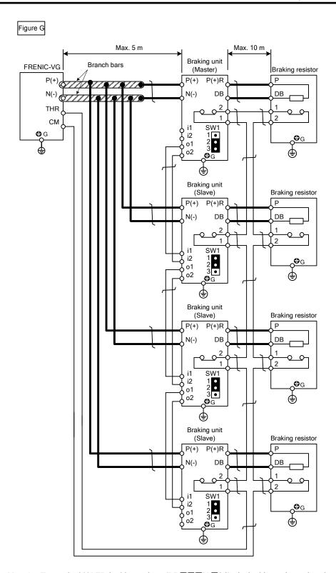
Note 1: To use the 20% ED braking resistor (DB DD DV-D2C), the braking unit requires the fan unit (BU-F).
