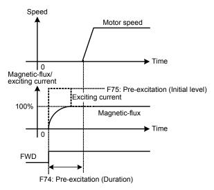
Under vector control without speed sensor and when H09 = 1 or 2 (Auto search is enabled), the data setting range is limited to 200 to 400%. Even if F75 is set at 100%, 200% applies.
