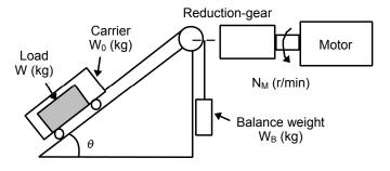
Figure 9.8 Inclined Lift Load
