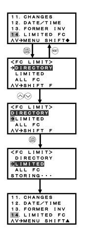
To display this menu screen, press the key in Running mode to switch to Programming mode.
