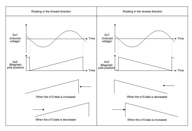
Figure 3.5-7 Adjustment of Magnetic Pole Position
