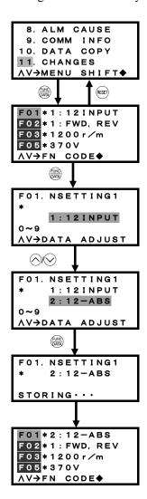
To display this menu screen, press the key in Running mode to switch to Programming mode.
