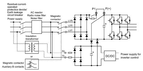
Figure 3.3-6 Connection Example of Residual-current-operated Protective Device (RCD)/ Earth Leakage Circuit Breaker (ELCB)
