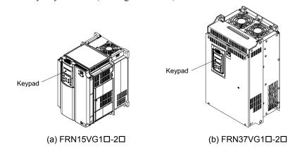
Figure 3.3-19 Mounting the Keypad Directly on the Inverter
