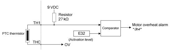
The warning temperature depends on a PTC thermistor and the resistor of the PTC thermistor changes drastically at the warning temperature. The activation (voltage) level is specified by this change of the resistor.
