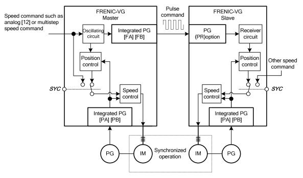
The complete synchronization ( $\pm$  2 pulses or less) is possible both in the application example 1 and 2 during both transient and steady states.
