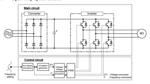
Figure 1.3.2 Open-loop Speed Control: Basic Architecture
