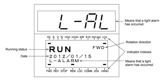
Figure 3.4-7 Display of Light Alarm
