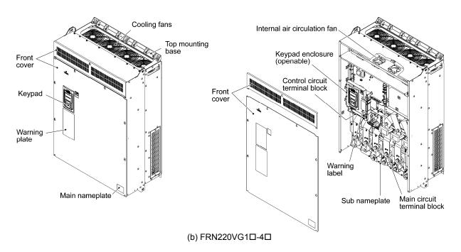
Figure 3.1-2 Outside and Inside Views of Inverters
