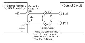
Figure 3.3-10 Example of Electric Noise Reduction
