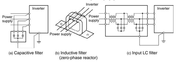
Figure A.10 Various Filters and their Connection
