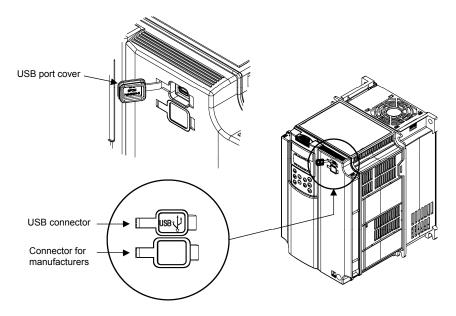
Figure 3.3-27 Connecting a USB Cable
