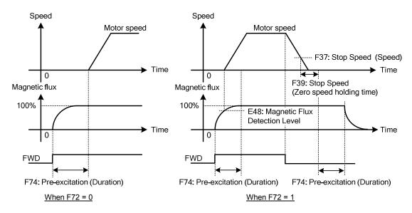
When F72 = 0, set the pre-excitation duration (F74) so that the motor starts rotating after the magnetic flux has been saturated (100%), as shown in the above graph.
