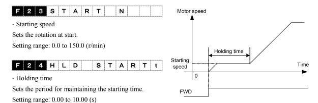
Note: The holding time is not activated when you switch between forward and reverse rotation. The acceleration time does not include the holding time.
