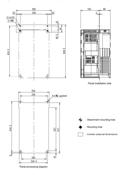
Figure 8.13 External Cooling Attachment External Dimensions
