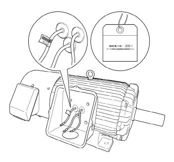
Figure 3.5-5 Magnetic Pole Position Offset Label Attaching Position Example
