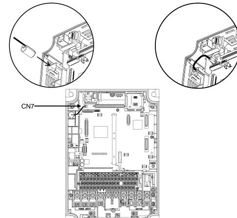
Figure 8.15 Battery Installed (22 kW or lower)
