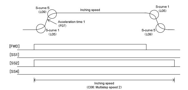
How to calculate acceleration/deceleration times and travel distance
