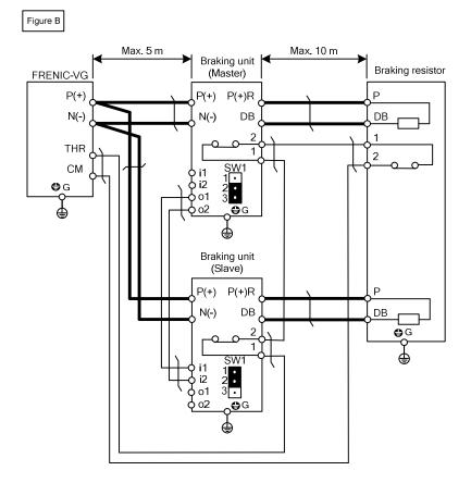
Note 1: To use the 20%ED braking resistor (DB \Bullet \Bullet V-\Bullet 2C), the braking unit requires the fan unit (BU-F).
