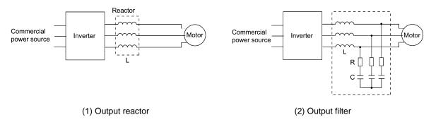
Figure C.3 Method to Suppress Surge Voltage
