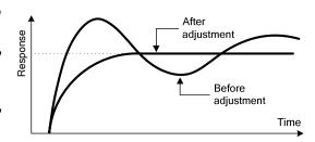
Follow the procedure below to adjust the response waveform.
