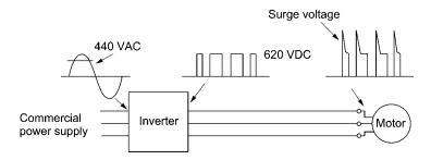
Figure C.1 Voltage Waveform of Individual Portions
