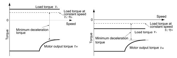
Figure 9.4 Example Study of Minimum Deceleration Torque (1)
