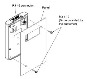
Figure 3.3-25 Mounting the Keypad
