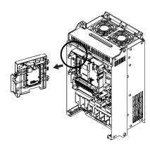
4 Connect the battery cable to the connector CN7 on the control printed board.
