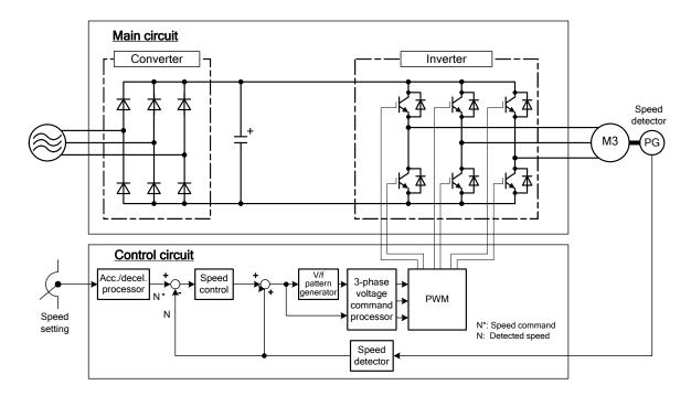
Figure 1.3.6 Slip Frequency Control Architecture
