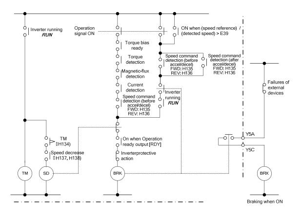
Servo locking function (braking not by a mechanical brake but by the inverter output torque) is also available. See the zero speed locking command in E01 to E13 "X function selection" for more details. We recommend to use the servo lock function not independently but together with a mechanical brake.
