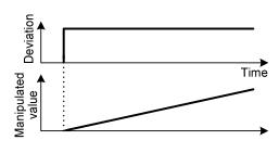
You can use I: integral time as a parameter to determine the effect of I control action. If you set a large integral time, you will have a slow response. A large integral time also decreases the repulsive force.
