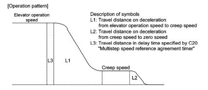
The estimated travel distance on deceleration appears on the "Option monitor 3, 4" on the LED monitor of the KEYPAD panel.
