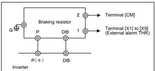
Figure 8.7 Braking Resistor (Standard Model) and Connection Example
