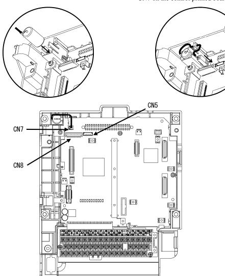
Figure 8.16 Battery Installed (30 kW or higher)
